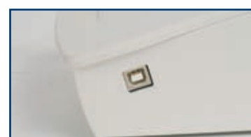
4 Connection to PC that allows : - Upgrade the TRS-5000. - Code reading. - Code store. - Code modification. - Database creation.
